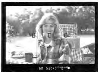
Partial metering circle
